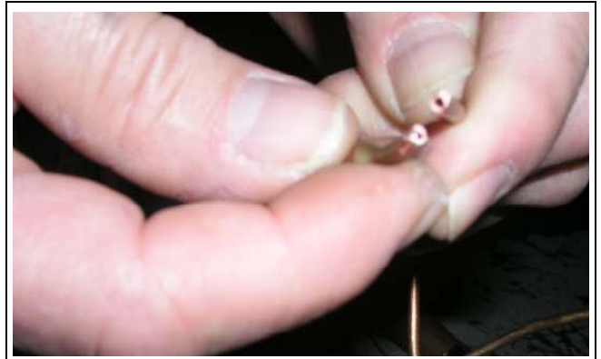
FIGURE 3: Cut Equalizer Tube Without Blockage
