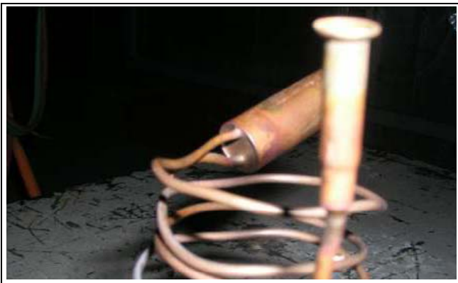
FIGURE 1: Original TXV Showing Equalizer Tube
