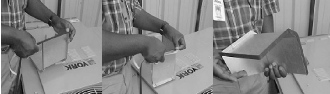
FIGURE 3 - GASKET STRIP APPLICATION
